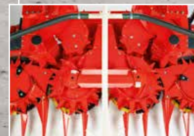
Optimum utilisation of the wide chopping drum is permitted through the enlarged intake channel. For this reason, the stepped feeder drums are located further to the outside.
