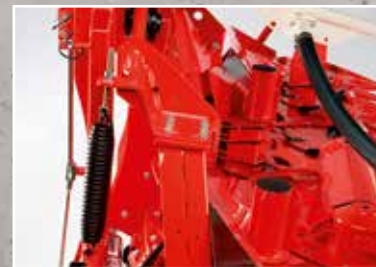
The mechanical lateral tilting frame is available as standard equipment.
