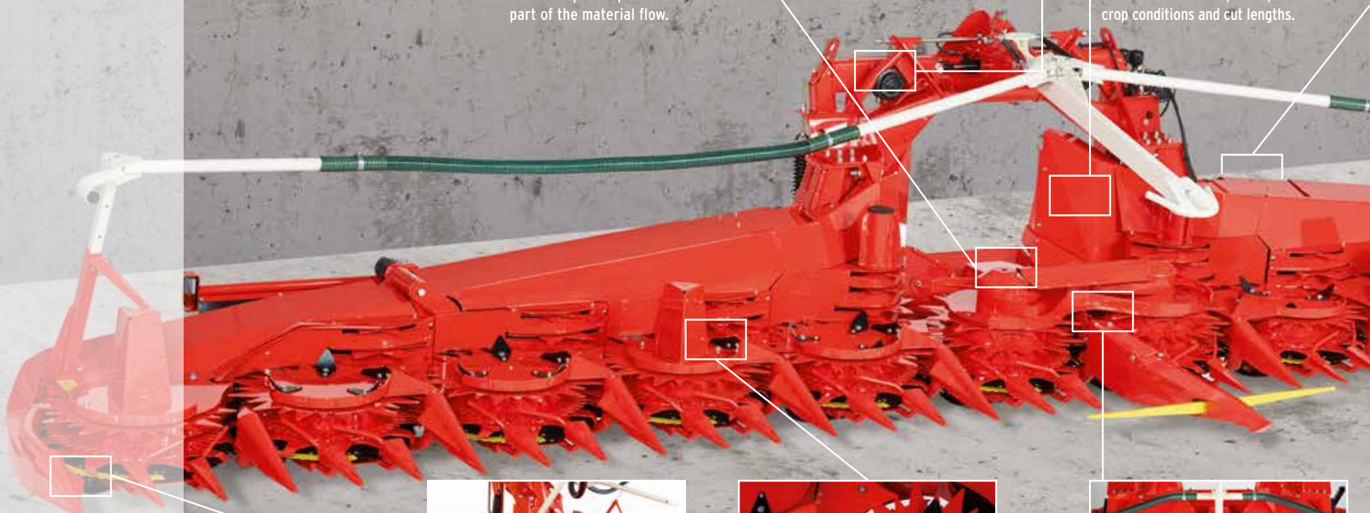
The mechanical lateral tilting frame is available as standard equipment.
